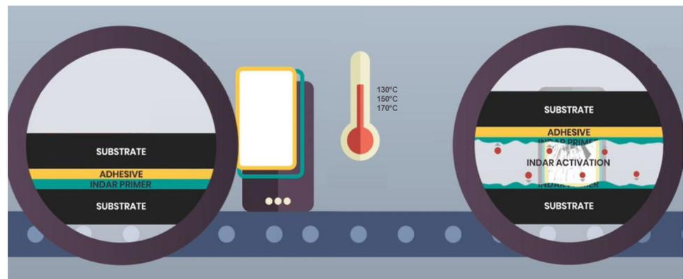
**Figure 11.** Schematic representation of the INDAR<sup>®</sup> debonding technology, reused with permission from [46].
