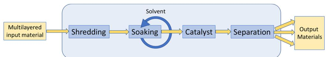
**Figure 12.** Schematic representation of the PolySep process.
