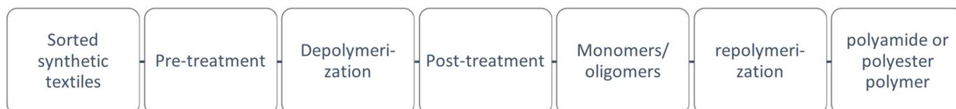
**Figure 6.** General process scheme for the recycling of synthetic fibres, such as polyamide and polyester, into the same synthetic fibres via monomer recycling.
