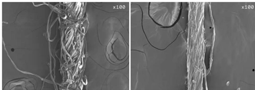
**Figure 3.** Microscopic image of cotton yarn, lengthwise, before (left) and after (right) one type of (tuneable) Clarus® fibre welding transformation by NFW [22]. Imparting these new tuneable morphologies gives CLARUS® yarns and fabrics new performance properties of increased durability, enhanced moisture wicking, and even new fabric construction options.
