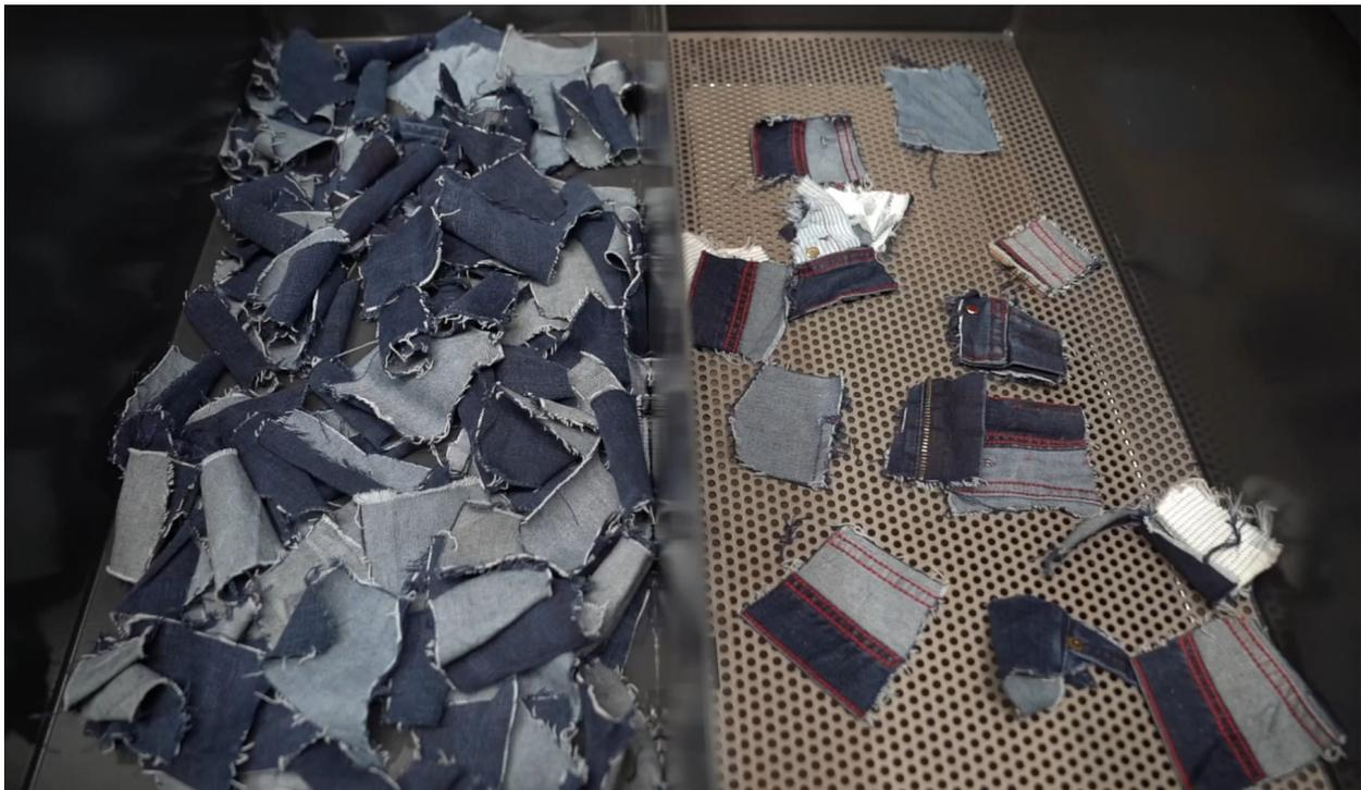
**Figure 8.** Clippings with trims (right) separated from untrimmed clippings (left) by Valvan’s Trimclean™ technology (<https://www.valvan.com/en/solutions/textile-sorting-recycling>).
